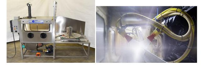
This equipment works well with powder-bed technologies by improving the overall surface finish significantly, while cleaning off the build material and eliminating the dust associated with other methods of build removal. They are available in both manual and fully automated systems in a variety of sizes, and can also be customized to your application.
